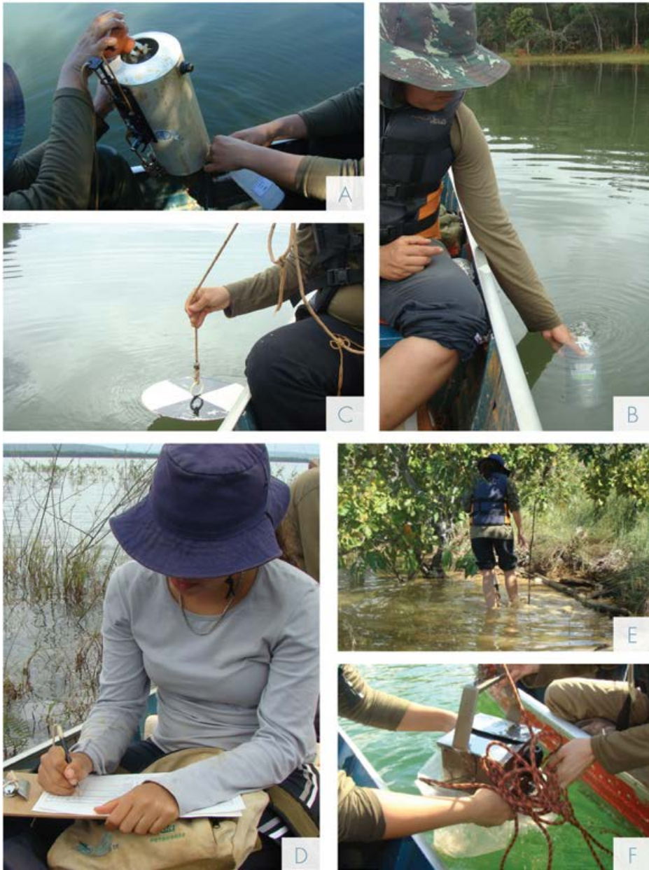
FIGURE 10. Reservoir sampling. Collecting water samples (A; B; C), applying the physical habitat protocol (D), collecting macroinvertebrates with a kick-net (E), and collecting sediment and macroinvertebrates with an Eckman-Birge dredge (F).
