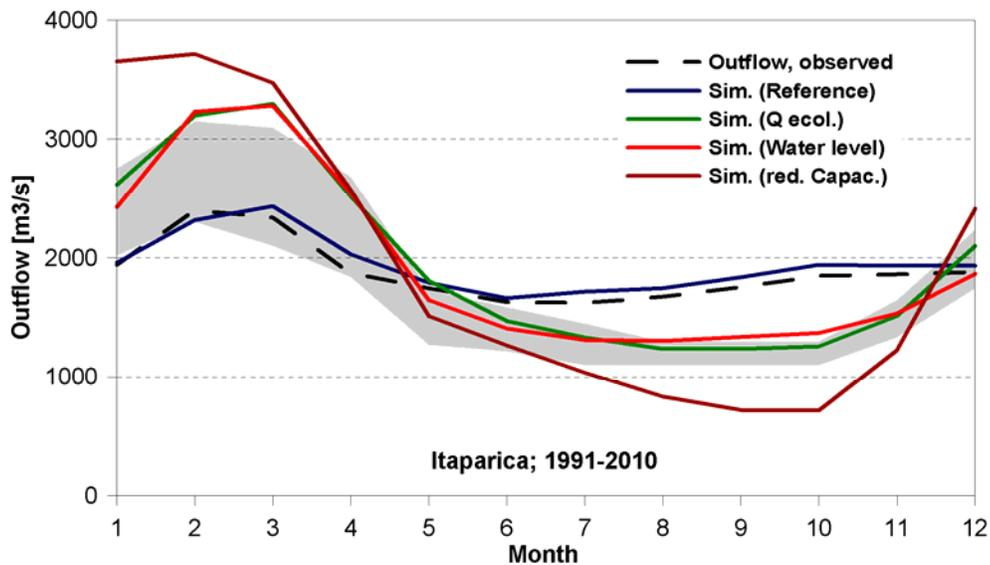
**Fig. 7: Mean monthly outflow Itaparica reservoir; grey shaded area: minimum discharge for normal and dry year (*hidrogramas ambientais*) according to project AIHA**
