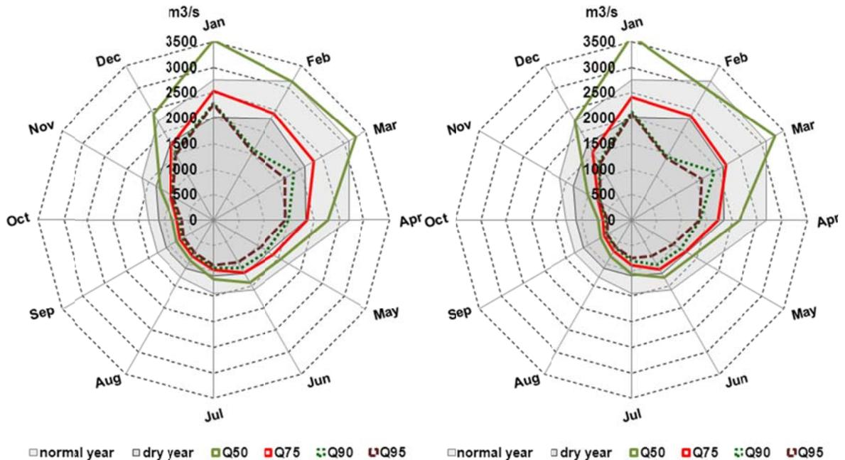
**Fig. 11: Monthly outflows (Q50, Q75, Q90 and Q95) Sobradinho reservoir (left) and Itaparica reservoir (right) for option “Reduced Capacity”; grey shaded areas: minimum discharge for normal and dry year (*hidrogramas ambientais*) according to project AIHA, years 1991-2010**
