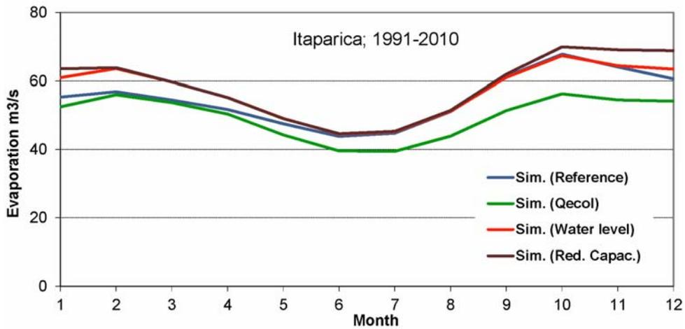
Fig. A2: Mean monthly evaporation rates Itaparica reservoir
