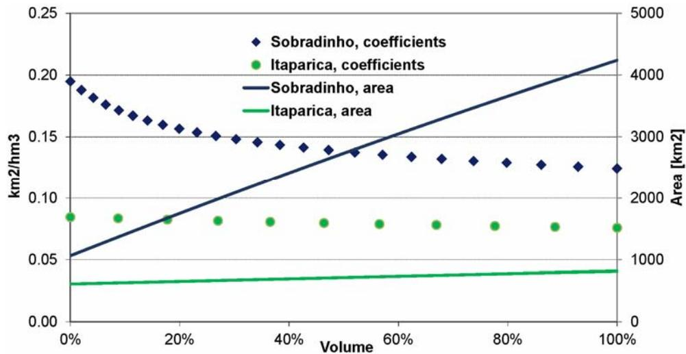
**Fig. 1: Relation of volumes (live capacity) to water surface area and to area-volume-coefficient for Sobradinho and Itaparica reservoirs**
