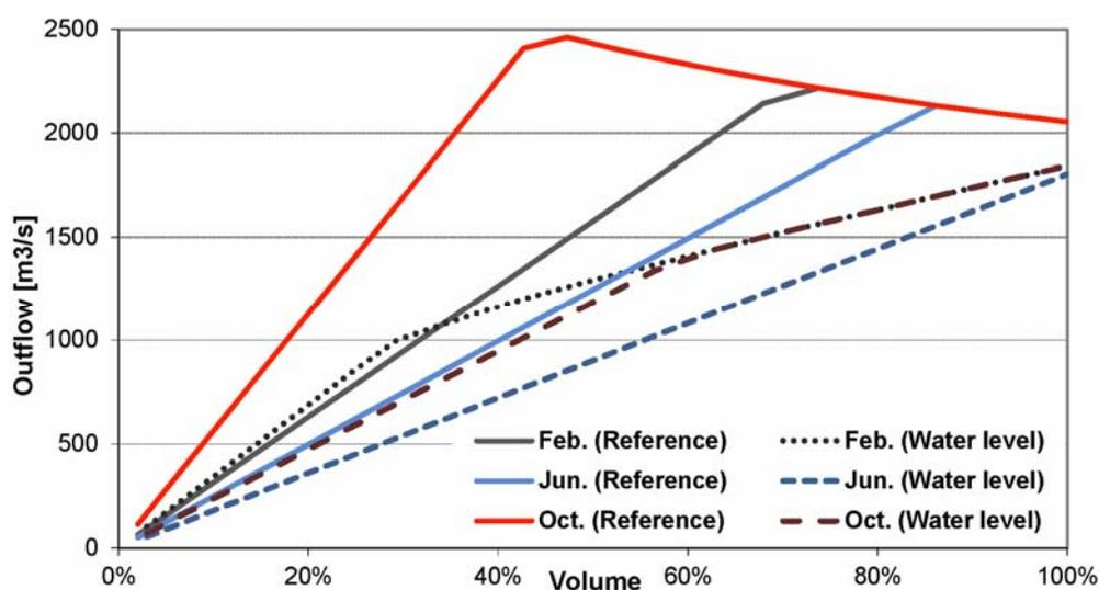
**Fig. 3: Rule curves for outflow Sobradinho reservoir, management options Reference (100%= 28 669 hm<sup>3</sup>) and Water level (100%= 19 479 hm<sup>3</sup>)**
