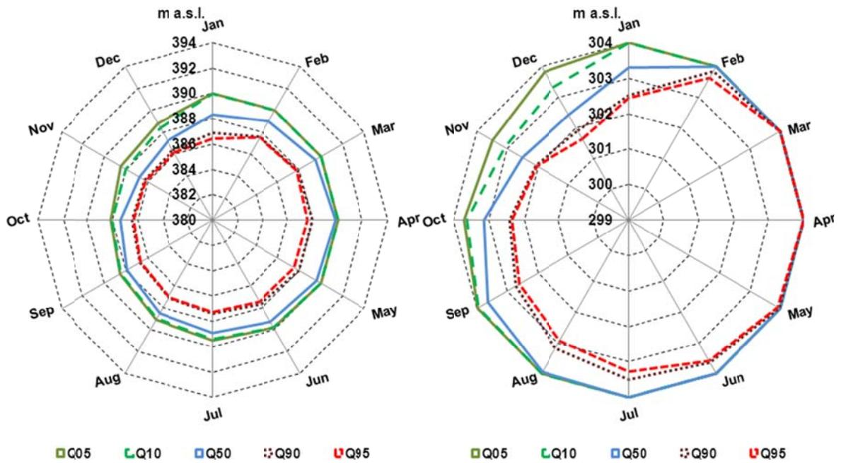
Fig. 14: Monthly water levels (Q05, Q10, Q50, Q90 and Q95) Sobradinho reservoir (left) and Itaparica reservoir (right) for option “Water level”, years 1991-2010
