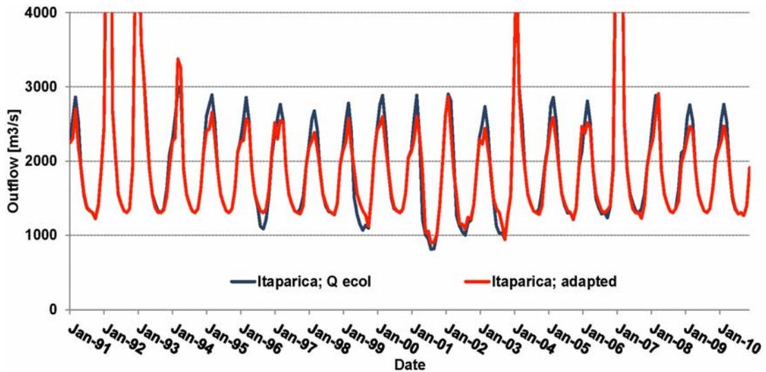
Fig. 18: Monthly outflow from Itaparica reservoir for option “Qecol.” for values according to project AIHA (*hidrogramas ambientais*) and for adapted minimum discharge
