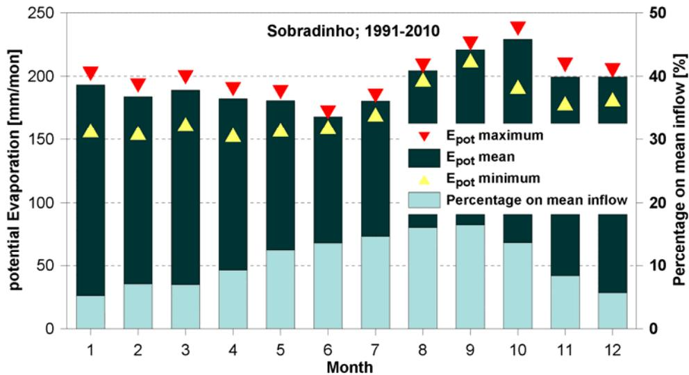
**Fig. 2: Minimum, mean and maximum monthly potential evaporation and the share of mean monthly evaporation on observed mean monthly inflow for Sobradinho reservoir**
