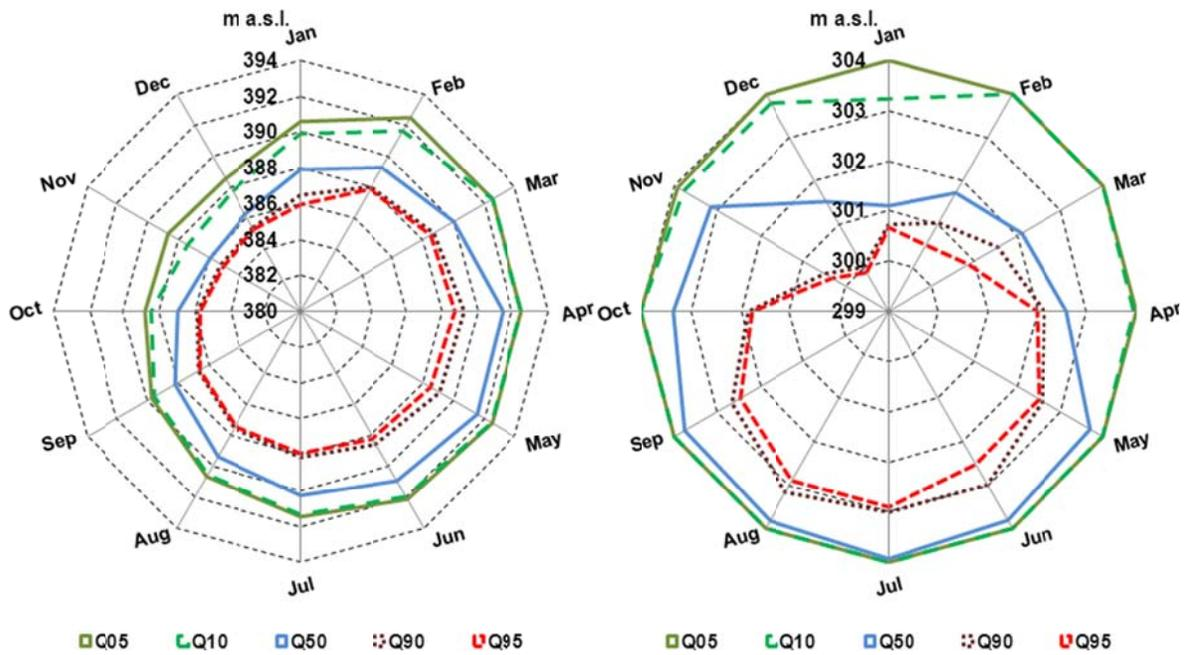
Fig. 12: Monthly water levels (Q05, Q10, Q50, Q90 and Q95) Sobradinho reservoir (left) and Itaparica reservoir (right) for “Reference”, years 1991-2010
