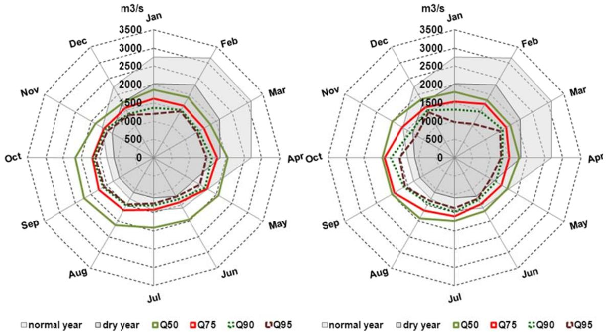
Fig. 8: Monthly outflows (Q50, Q75, Q90 and Q95) Sobradinho reservoir (left) and Itaparica reservoir (right) for “Reference”; grey shaded areas: minimum discharge for normal and dry year (*hidrogramas ambientais*) according to project AIHA, years 1991-2010
