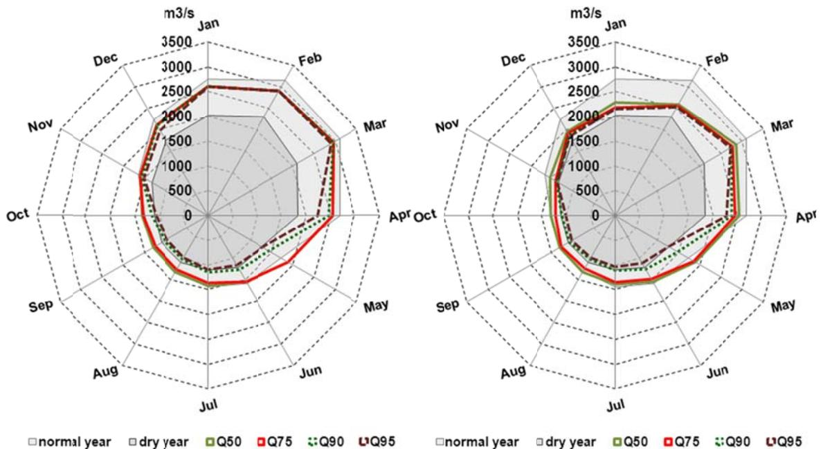
Fig. 9: Monthly outflows (Q50, Q75, Q90 and Q95) Sobradinho reservoir (left) and Itaparica reservoir (right) for option “Ecological Discharge”; grey shaded areas: minimum discharge for normal and dry year (*hidrogramas ambientais*) according to project AIHA, years 1991-2010
