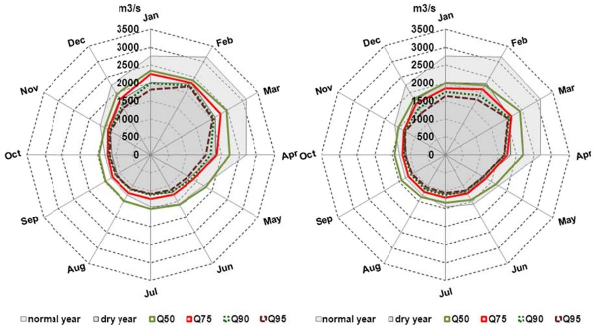
**Fig. 10: Monthly outflows (Q50, Q75, Q90 and Q95) Sobradinho reservoir (left) and Itaparica reservoir (right) for option “Water level”; grey shaded areas: minimum discharge for normal and dry year (*hidrogramas ambientais*) according to project AIHA, years 1991-2010**
