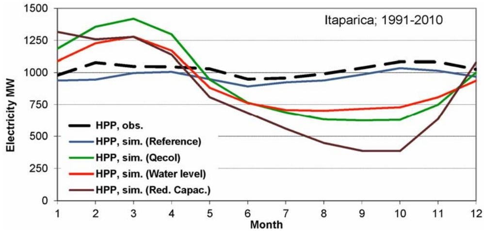
Fig. A4: Mean monthly electricity generation Itaparica reservoir
