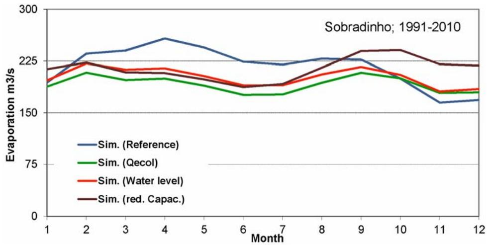
Fig. A1: Mean monthly evaporation rates Sobradinho reservoir
