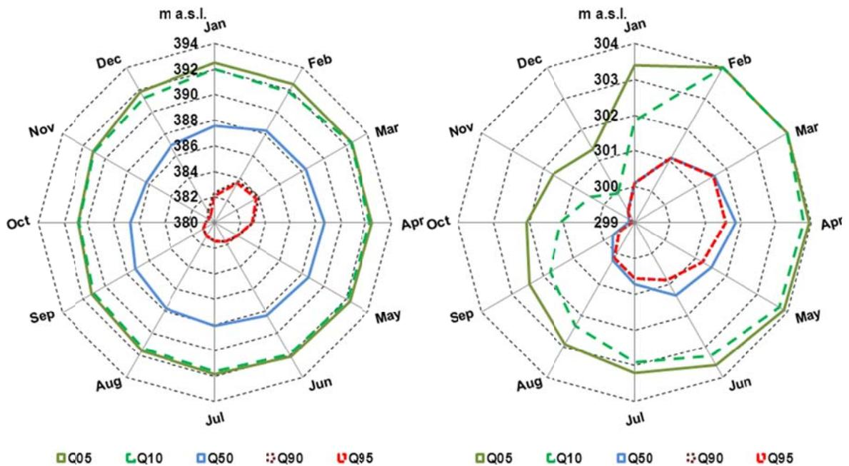
Fig. 13: Monthly water levels (Q05, Q10, Q50, Q90 and Q95) Sobradinho reservoir (left) and Itaparica reservoir (right) for option “Ecological Discharge”, years 1991-2010
