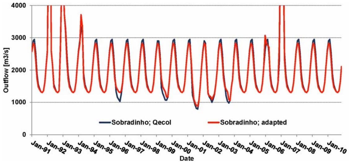
Fig. 16: Monthly outflow from Sobradinho reservoir for option “Qecol.” for values according to project AIHA (*hidrogramas ambientais*) and for adapted minimum discharge
