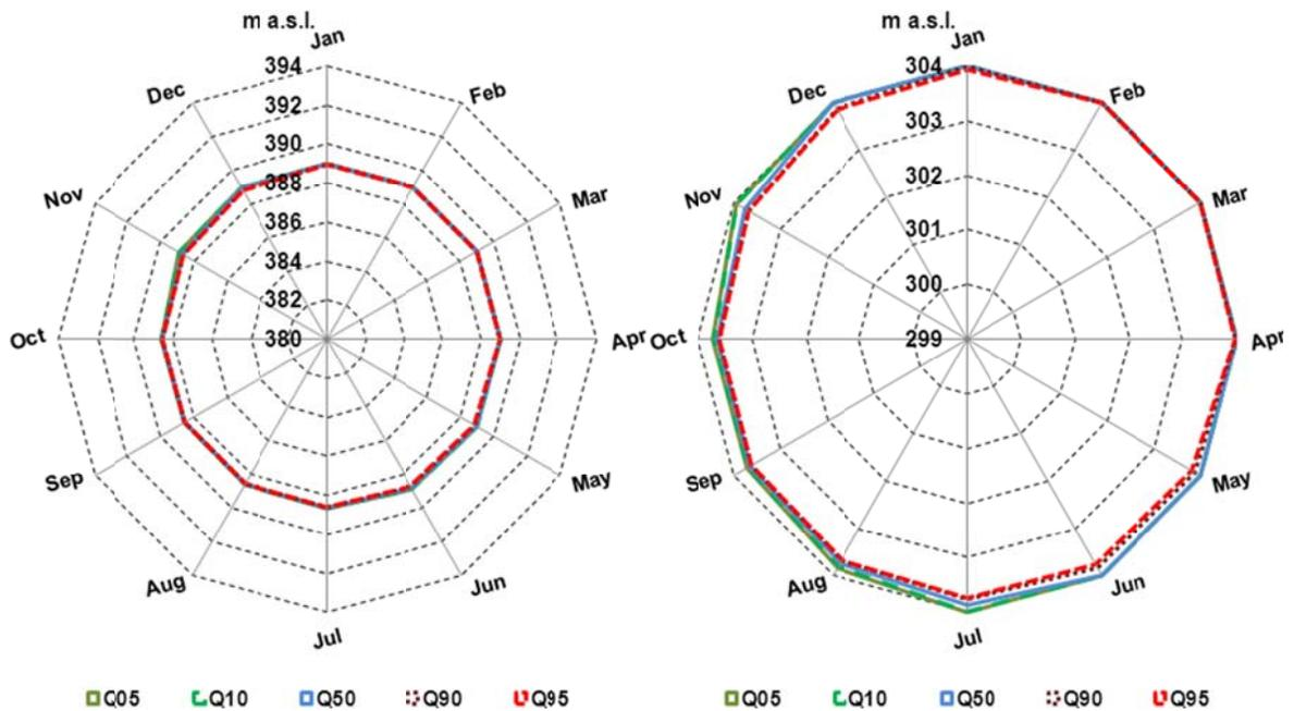
Fig. 15: Monthly water levels (Q05, Q10, Q50, Q90 and Q95) Sobradinho reservoir (left) and Itaparica reservoir (right) for option “Reduced Capacity”, years 1991-2010
