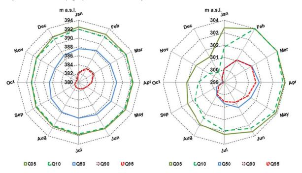
Fig. 13: Monthly water levels (Q05, Q10, Q50, Q90 and Q95) Sobradinho reservoir (left) and Itaparica reservoir (right) for option "Ecological Discharge", years 1991-2010
