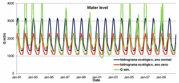
Fig. A10: Monthly outflow Itaparica reservoir for option "Water level"; minimum discharge for normal and dry year (*hidrogramas ambientais* according to project AIHA)
