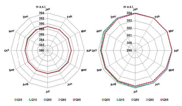
Fig. 15: Monthly water levels (Q05, Q10, Q50, Q90 and Q95) Sobradinho reservoir (left) and Itaparica reservoir (right) for option "Reduced Capacity", years 1991-2010
