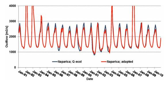
Fig. 18: Monthly outflow from Itaparica reservoir for option "Qecol." for values according to project AIHA (*hidrogramas ambientais*) and for adapted minimum discharge
