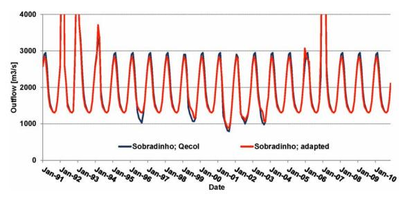
Fig. 16: Monthly outflow from Sobradinho reservoir for option "Qecol." for values according to project AIHA (*hidrogramas ambientais*) and for adapted minimum discharge
