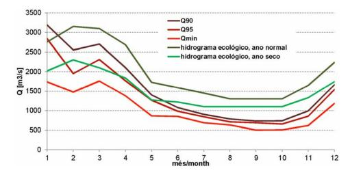
Fig. A6: Discharge at gauge Xingó, naturalized flows according to ONS (1931-2010); minimum discharge for normal and dry year (*hidrogramas ambientais* according to project AIHA)
