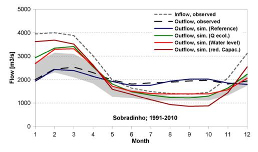
Fig. 6: Mean monthly flows for Sobradinho reservoir; grey shaded area: minimum discharge for normal and dry year (*hidrogramas ambientais*) according to project AIHA
