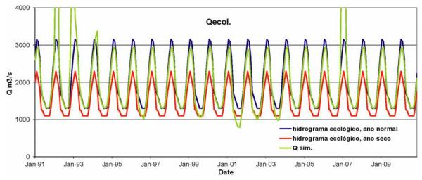
Fig. A7: Monthly outflow Sobradinho reservoir for option "Qecol."; minimum discharge for normal and dry year (*hidrogramas ambientais* according to project AIHA)
