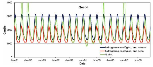
Fig. A8: Monthly outflow Itaparica reservoir for option "Qecol."; minimum discharge for normal and dry year (*hidrogramas ambientais* according to project AIHA)
