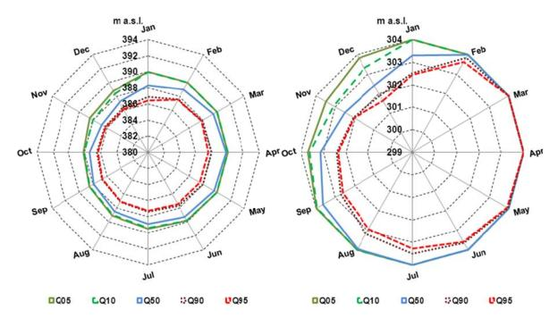
Fig. 14: Monthly water levels (Q05, Q10, Q50, Q90 and Q95) Sobradinho reservoir (left) and Itaparica reservoir (right) for option "Water level", years 1991-2010
