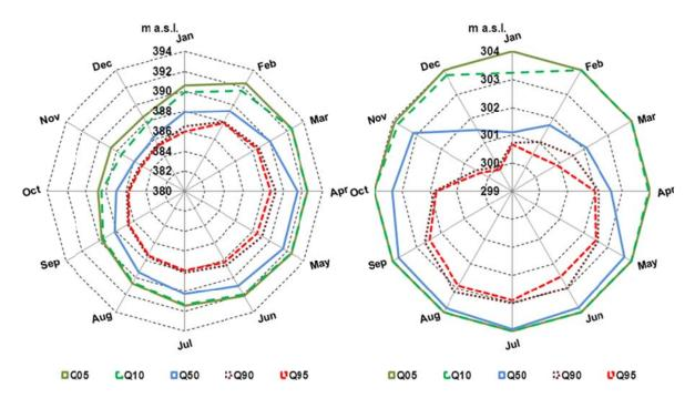
Fig. 12: Monthly water levels (Q05, Q10, Q50, Q90 and Q95) Sobradinho reservoir (left) and Itaparica reservoir (right) for "Reference", years 1991-2010
