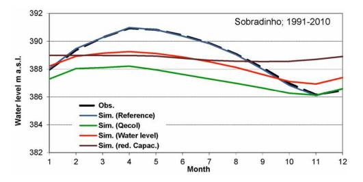
Fig. 4: Mean monthly water levels Sobradinho reservoir
