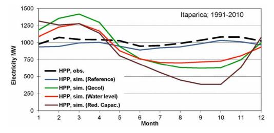
Fig. A4: Mean monthly electricity generation Itaparica reservoir
