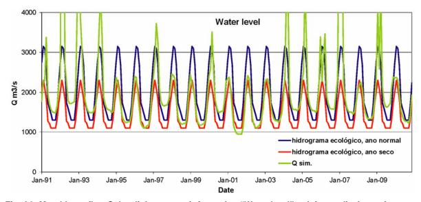
Fig. A9: Monthly outflow Sobradinho reservoir for option "Water level"; minimum discharge for normal and dry year (*hidrogramas ambientais* according to project AIHA)
